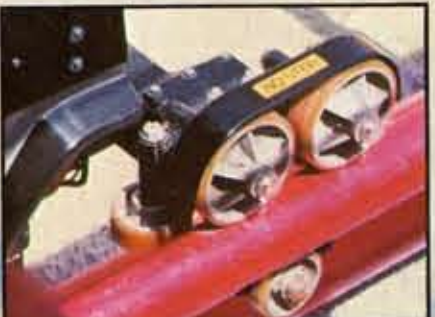
Small rollers keep coaster on the tracks.
